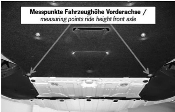
**Attachment 8 – Trimming of front underbody**
